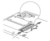
Figure 4-11 Removing a Memory Upgrade Module
